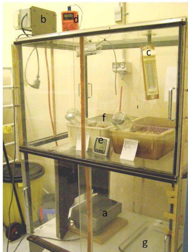
Figure 3.2.3.1.a The heating chamber used for the heating experiments. This chamber was equipped with a heater (EWT heater, Model 01S, Australia) (a), a universal programming controller (b) (R&H Wholesale (SA) Pty. Ltd., Australia), mercury thermometer (c), digital thermometer (d & e), animals cages (f) and glass container containing water to maintain optimum humidity (g).
