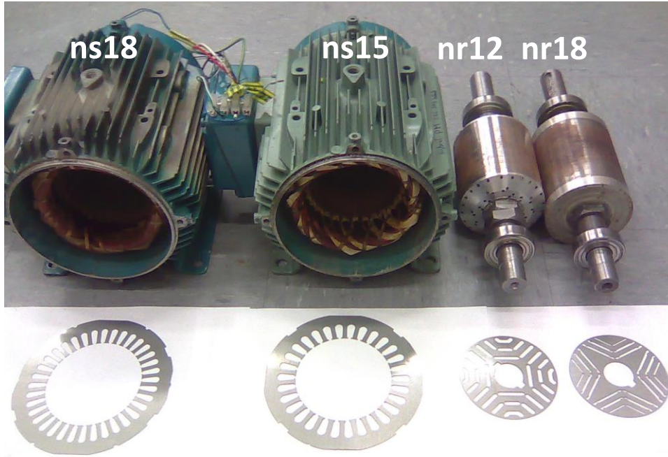
Figure 4-9: The ns18 and ns15 stators, and nr12 and nr18 rotors from left to right
