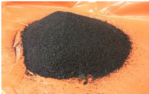
Fig.4.51 Granulated lead smelter slag (GLSS) used in UHPFRC
