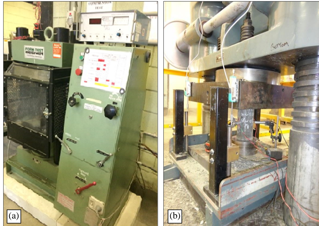
Fig.4.9 (a) Testing of cylinders using Seidner compression machine (b) Test set up and instrumentation by Amsler for UHPFRC specimens
