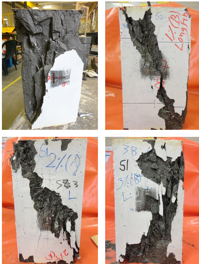
Fig.5.66 Failure pattern of 5D fiber specimens (Test series -2)
