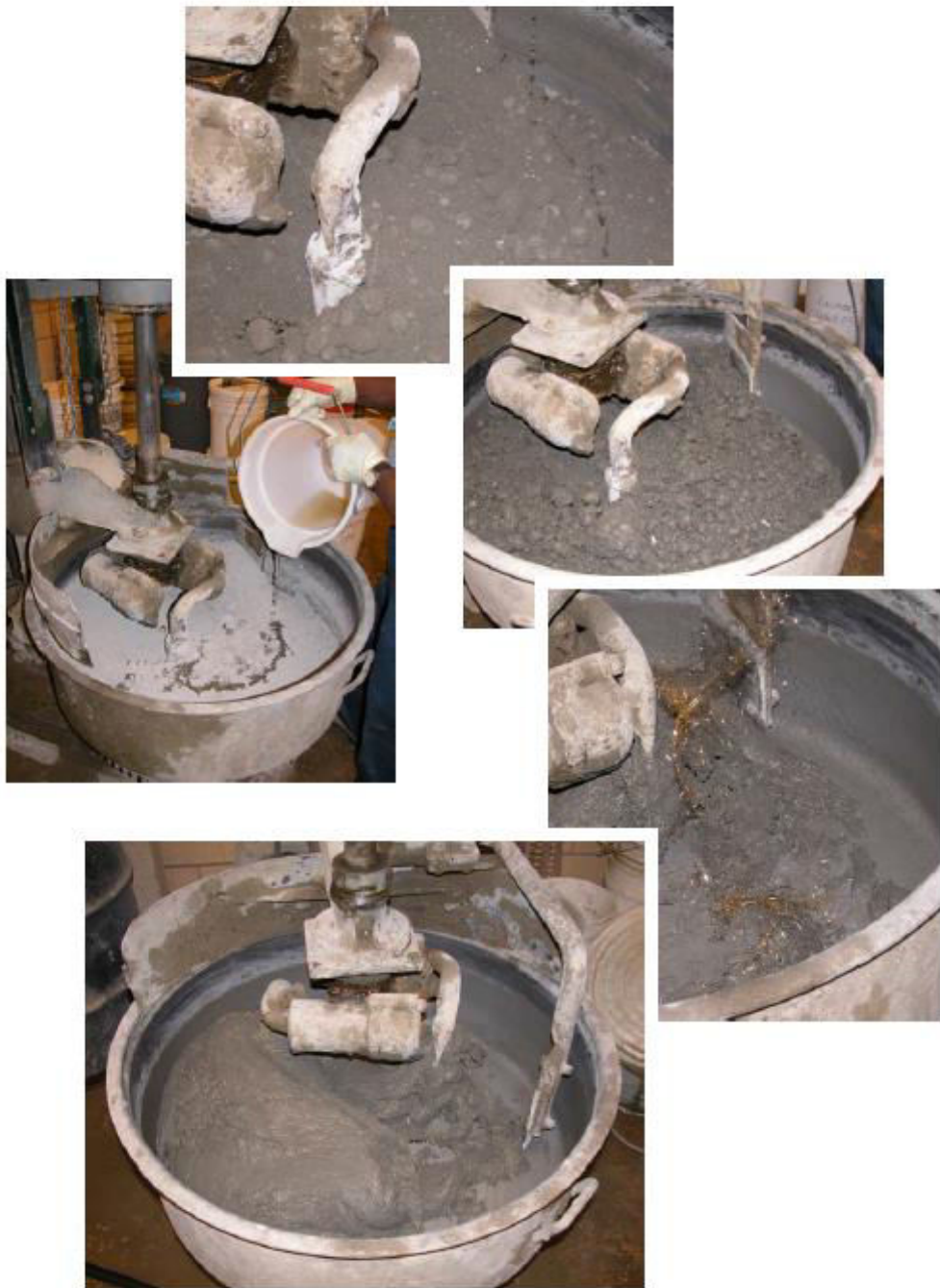
Fig.2.3 Mixing procedure of UHPC (Graybeal, 2005)
