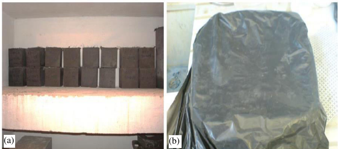
Fig.2.4 Curing process (a) Specimen stored at 20 0 C (b) The specimens cured with steam (Camacho Torregrosa, 2014).
