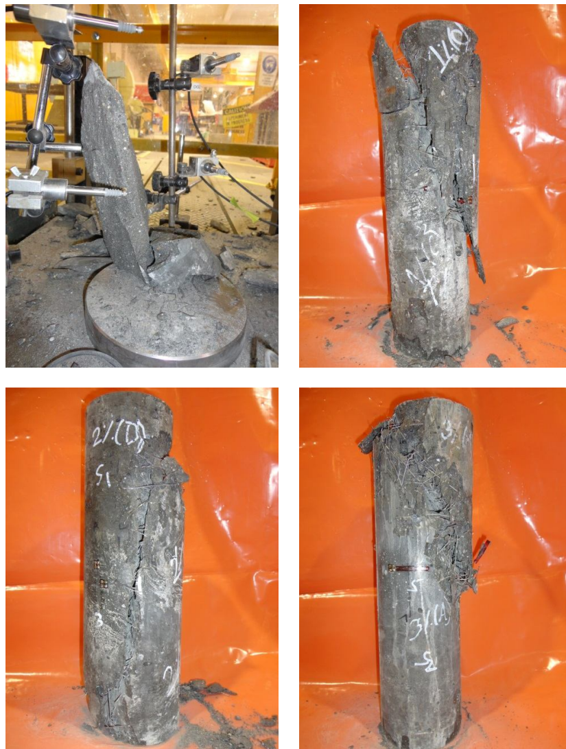
Fig.5.67 Failure pattern of 4D fiber specimens (Test series -3)
