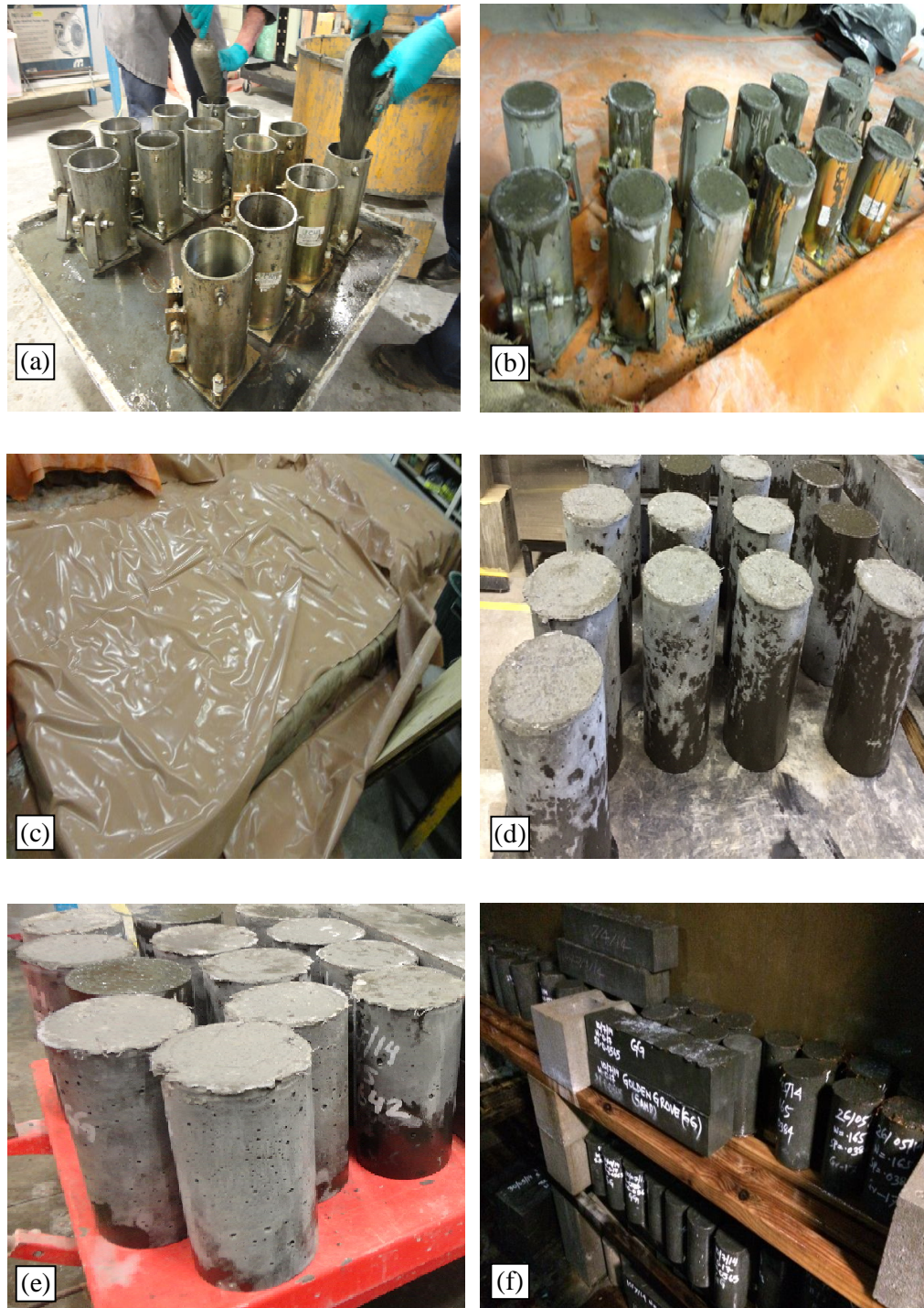
Fig.4.4 (a) Cylinder being filled (b) Cylinder placed on level surface after filled (c) Specimen put on the table after demoulding (d) Marked the specimens (e) Put wet hessian and plastic sheets after demoulding (f) Curing the specimens in fog room
