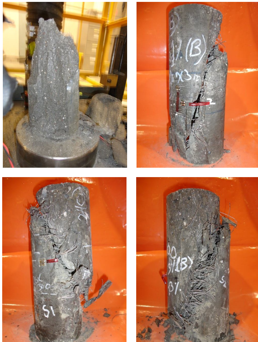
Fig.5.68 Failure pattern of 4D fiber specimens (Test series -4)
