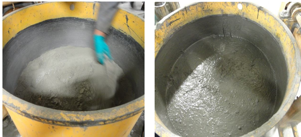
Fig.4.3 (a) Mixing of constituents of UHPC (b) After mixing of UHPC
