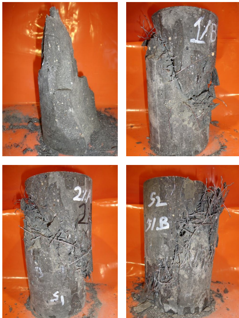
Fig.5.63 Failure pattern of 4D fiber specimens (Test series -1)
