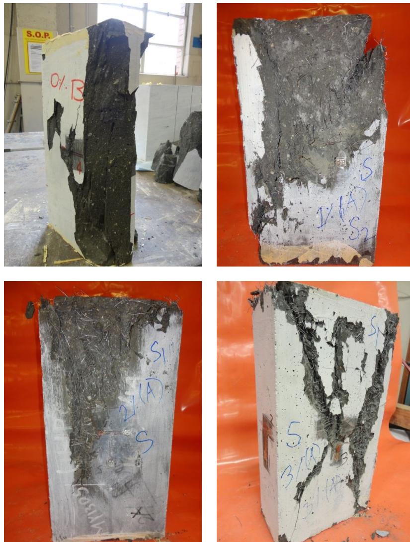
Fig.5.65 Failure pattern of 3D fiber specimens (Test series -2)
