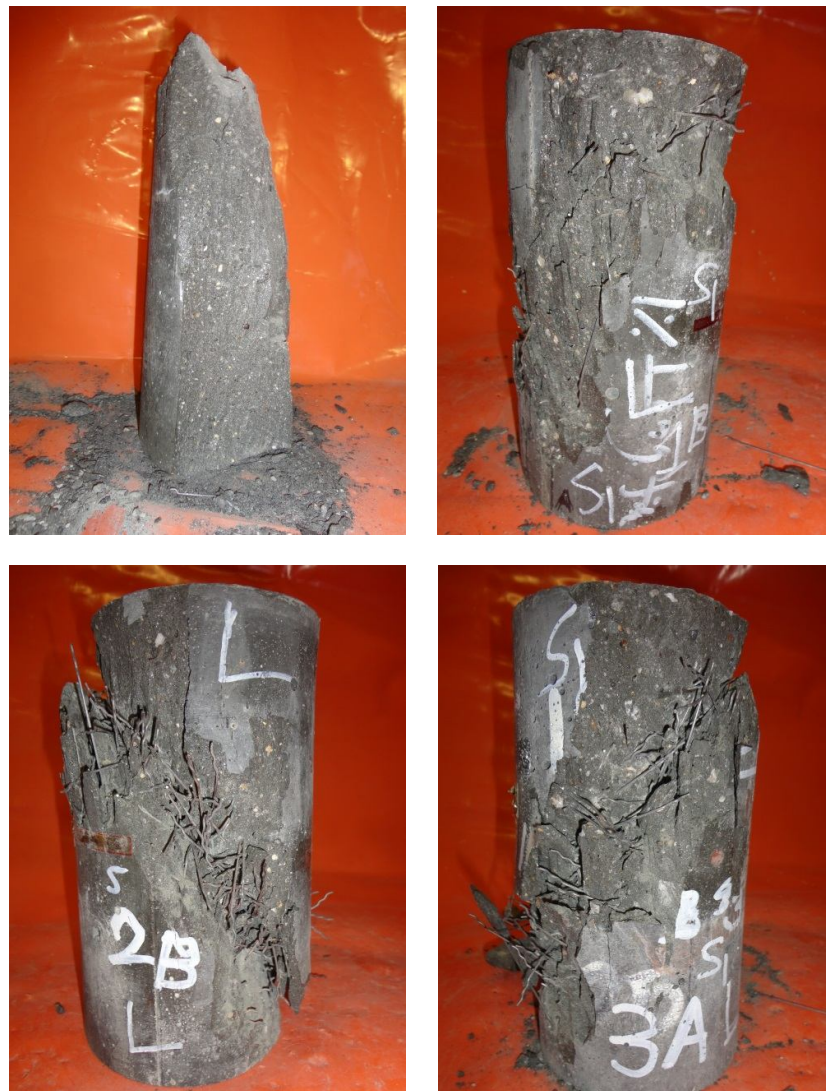
Fig.5.64 Failure pattern of 5D fiber specimens (Test series -1)
