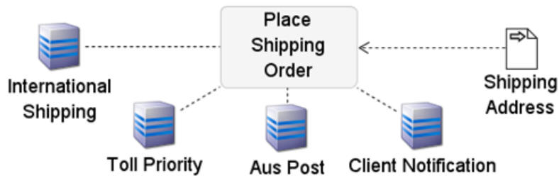
Figure 5.2: Configurable resources and data objects mapped to a BPMN activity
