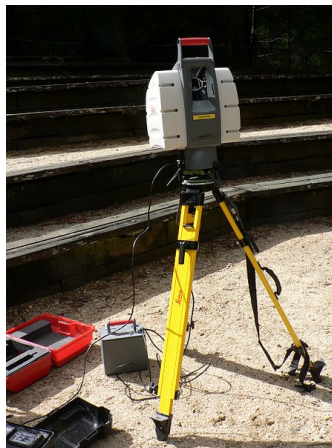
FIGURE 3.1: Example of terrestrial LIDAR scanner. Source: Wikimedia Commons .
