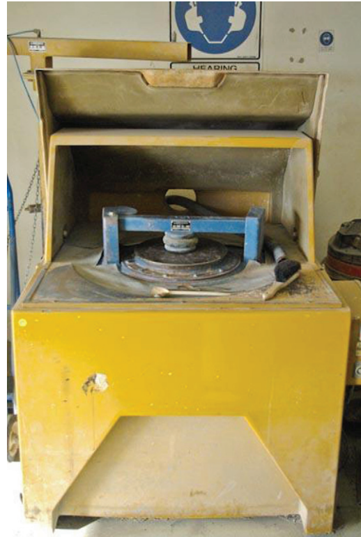
Figure 1. Mechanical grinder used to grind the coal ash
