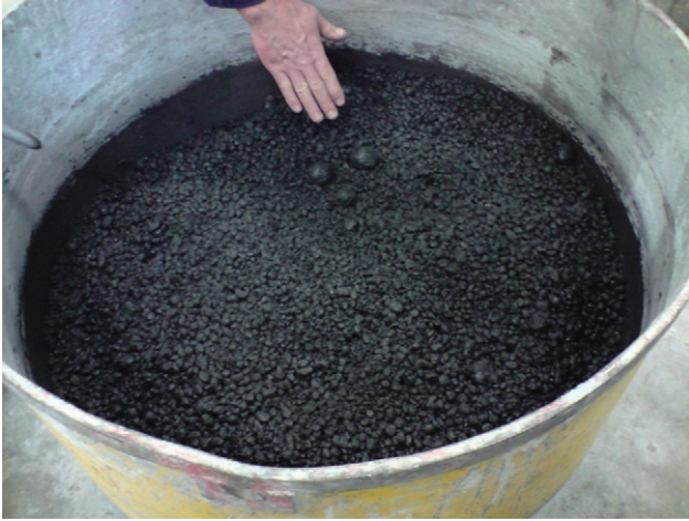
Figure 5. Balls of wet paste formed during the mixing of BA-based GPC
