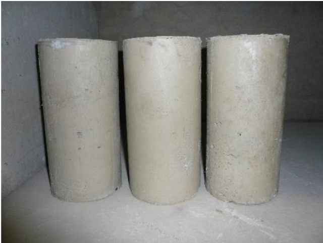
Fig. 5. Appearances of F100-0.25, F100-0.3 and F100-0.35 series: no visible efflorescence.
