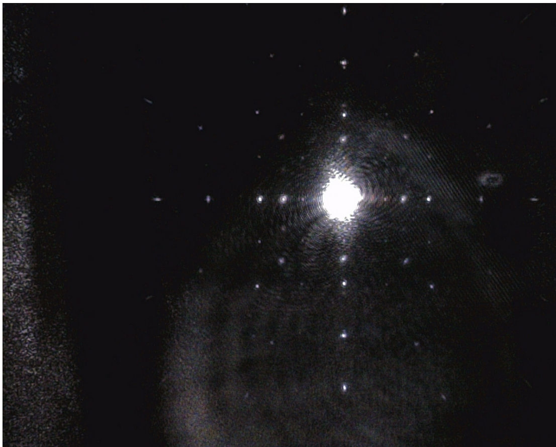
Figure G.4: Fourier transform of pump beam observed with the USB microscope when the HR mirror front surface is at the pump waist.
