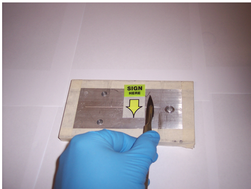
Figure B.2: Mounting the IR-Photonics fibre and creating incisions prior to cleaving.
