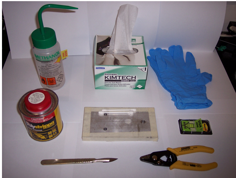
Figure B.1: Tools used for cleaving the IR-Photonics fibre. Clockwise from top-left: methanol, lint-free tissues, protective gloves, “Post-it” sticky flags, fibre stripper, scalpel, paint stripper, aluminium block and cotton swabs.
