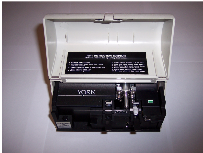
Figure B.4: Fibre in York cleaver with tissue on it. Clamps are in the open position.
