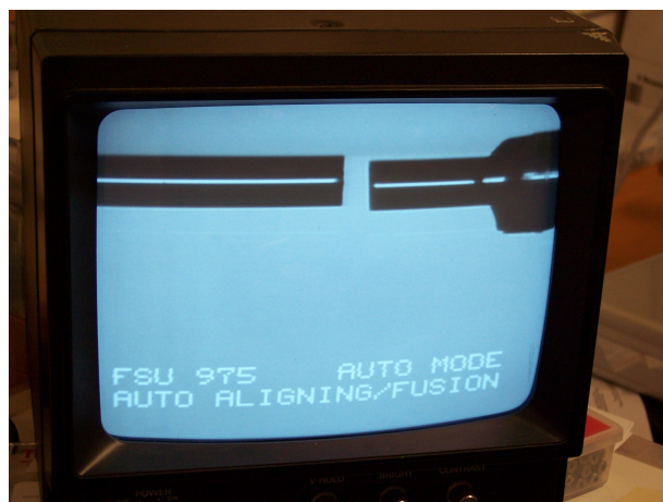
Figure B.6: Inspecting the fibre tip using a fibre splicer. The fibre on the left has an almost straight cleave, while the one on the right has an angled cleave.
