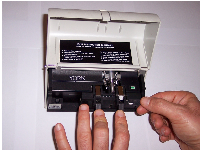
Figure B.5: Cleaving with the York cleaver when manually clamping the fibre. Leftmost lever is the “cleave” lever, two middle levers are the clamping levers and the rightmost lever is the “tension release” level.
