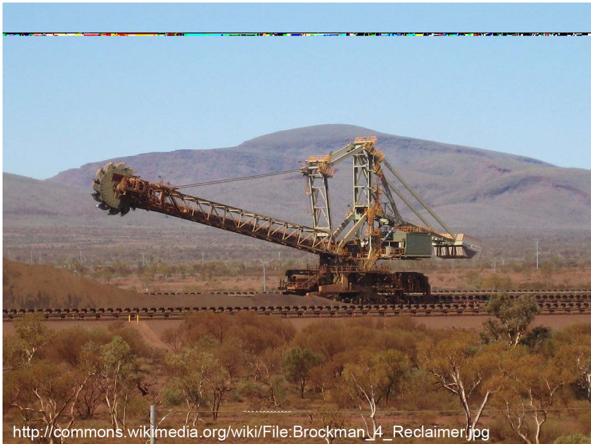
Fig. 2.2 A rail mounted BWR operated at the Brockman 4 mine in the Pilbara region of Western Australia. Image source: Wikipedia, under GNU Free Documentation Licence.
