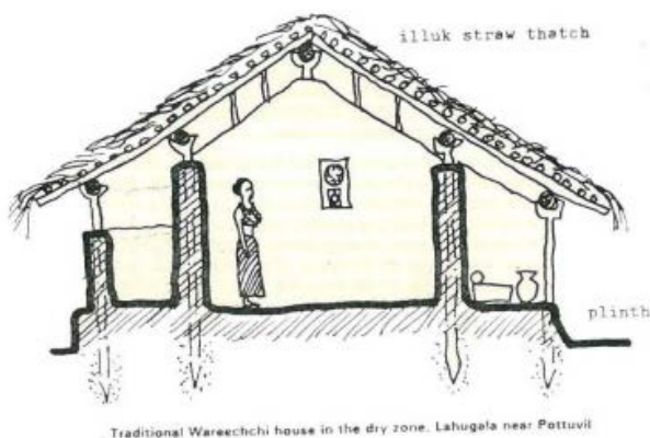
Figure 7.43 Traditional Dry Zone Housing Design (Sonya Redman, a Study of Support-based Housing and Community Participation in the Million Houses Programme, Sri Lanka 1977-1989 , a research report submitted for the Byera Hadley Student Travel Scholarship, (2005), 52, accessed on September 3, 2015, http://architectureinsights.com.au/media/uploads/resources/FINAL_MILLION_HOUSES_PROGRAMME_Sonya_Redman.pdf .)
