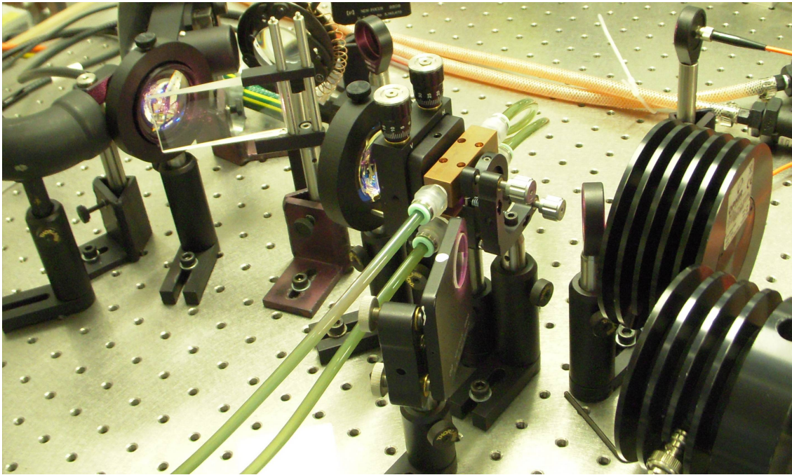
Figure 2.3: Schematic (top) and photo (bottom) of the initial Tm:YAlO 3 laser. The laser crystal is held within the copper cooling blocks.
