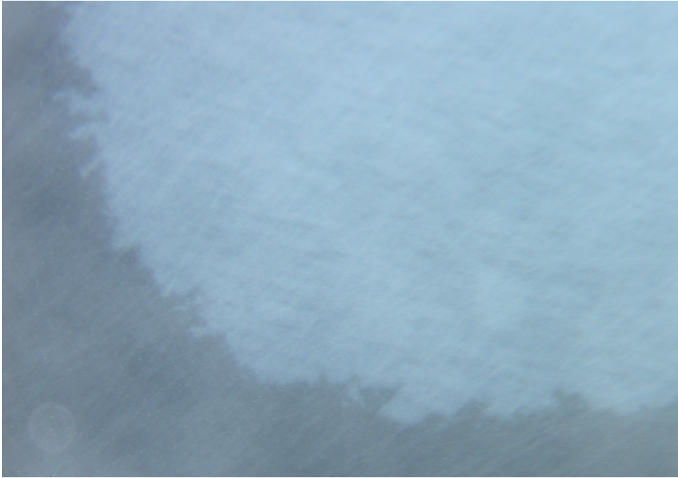
Figure 6.19: Microscope image of the hazy region in the diffusion bond.
