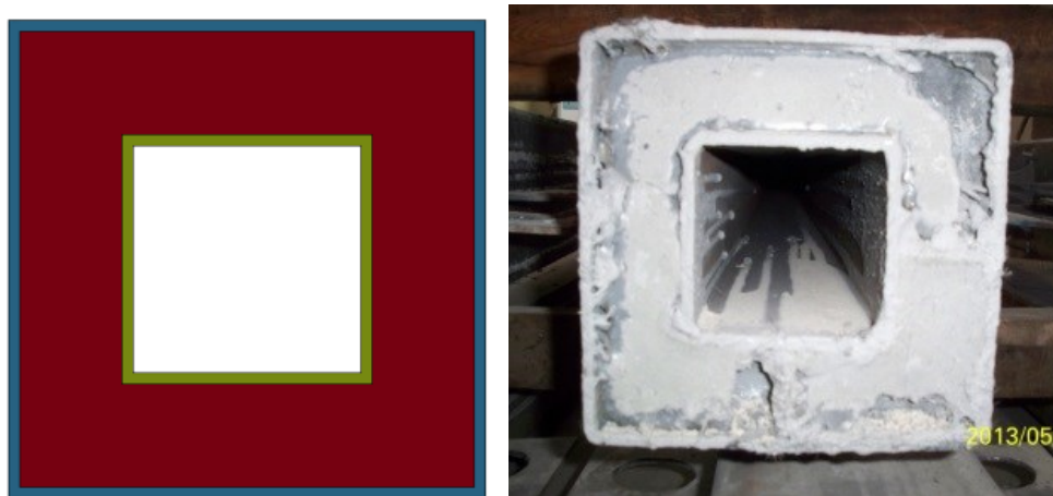
Fig. 2: Square cross section of the numerical model (left) and the actual column (right)
