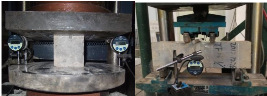
Fig. 3: Concrete compression test (left) and flexural tensile test (right)
