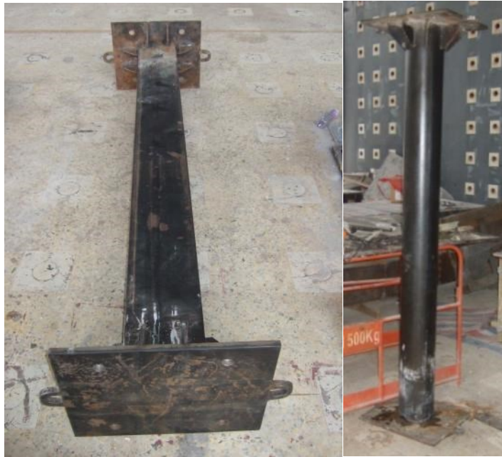
Fig. 1: Square (right) and Circular (left) CFST specimens
