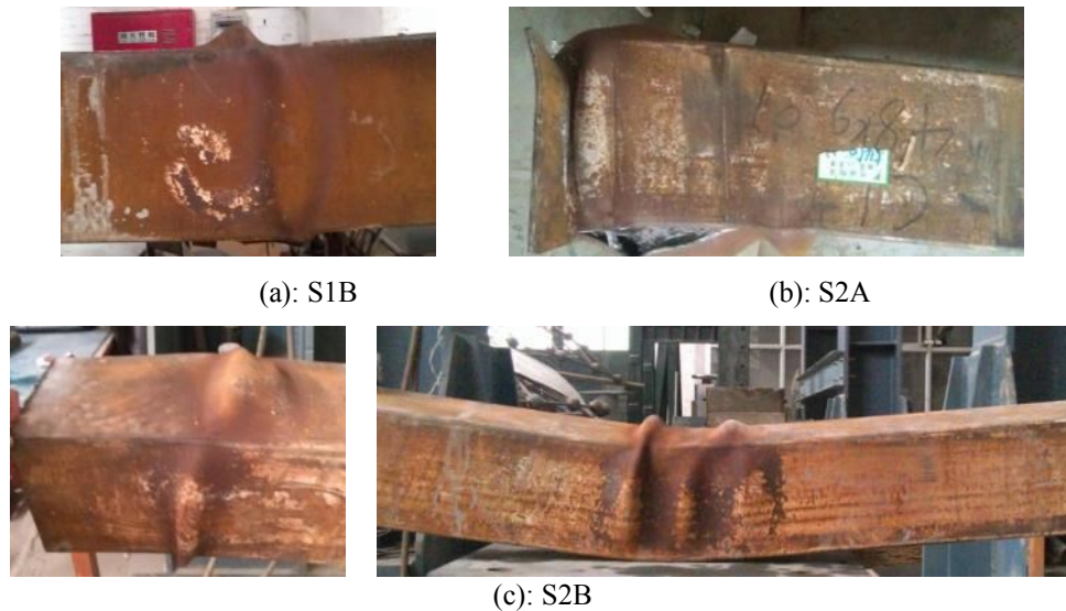
Fig. 22: Failure modes of square specimens
