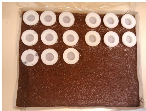
Fig. A5.4 DGT deployment in a soil test
