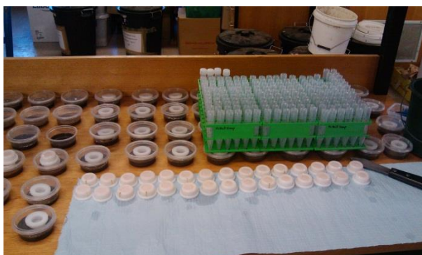
Fig. A5.5 Dismantling the DGT device and elution of the MAF gel
