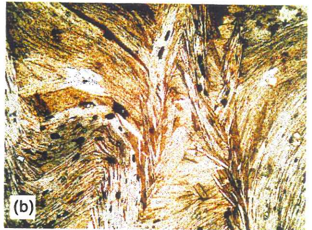
Fig. 5 - Thin section photos showing asymmetrically micro-folded slaty cleavage with wavelengths of (a) 3 mm and (b) 1 mm, developed within biotite rich metapelitic unit 200 m north of Sprigg Inlet, within the SISZ. Plane polarized light. Field of view is 4mm.
