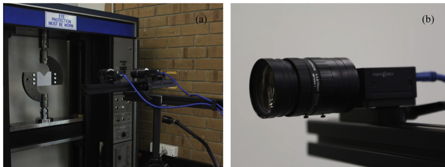
Fig. 4. (a) Experimental set up for the measurement of in-plane strain at the free surface of the specimen; (b) digital camera of the Vic-3D adopted in this work.
