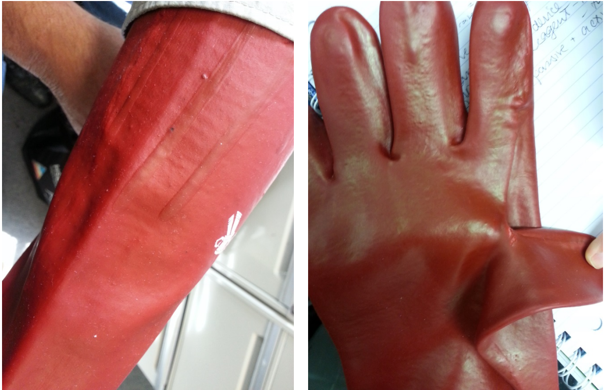
Photos showing PVC gloves (Excalibur) with running of coating (left) and tearing near the thumb (right) despite being new and unused.
