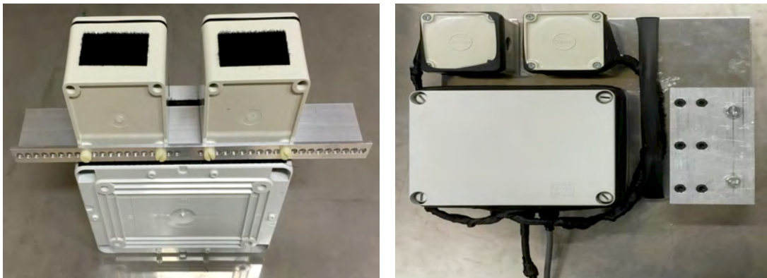
Fig. 4.24 Mounting configurations developed to control the spacing between the instrument sampling windows. The left configuration is light weight and suitable for balloon deployment and the right configuration is more sturdy, as required for deployment on a tower.
