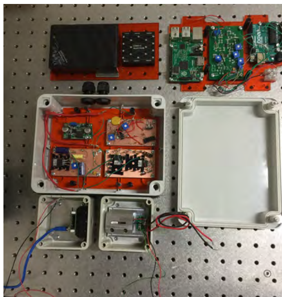
Figure 2. Digital holographic imaging system in designed enclosure. From top left to bottom right the following modular components are shown; external hard drive storage, computing and control systems, power regulation and pulsing circuitry, camera with optional optical filter and adjustable laser diode mount.
