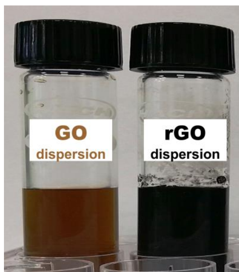
Supplementary Figure 4-1. GO (left) and rGO (right) dispersions.
