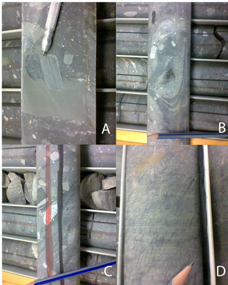
Figure 15 A) shows sand and shale clasts being deposited on a shale layer B) sand and shale mixing C) abundant clasts among shale and sand layers D) shear fabric.
