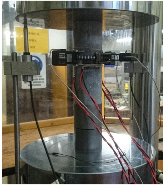
Fig. 3 Cylindrical specimen before deformability testing commenced with strain gauges and extensometers
