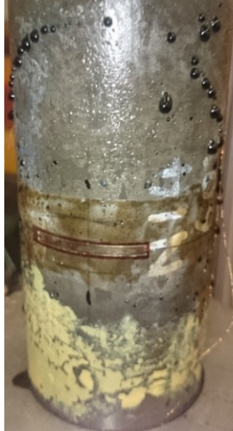
Fig. 10 Fracturing of specimen number 14 with dip angle of 60^\circ , under normal faulting conditions (initial normal stress of approximately 10 MPa, and initial shear stress of approximately 1.5 MPa)
