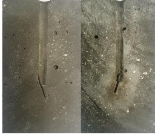
Fig. 2 Prototype specimen cut in half along the axis of the borehole, showing a 75° pre-existing circular notch at the bottom of the borehole section (on both halves)
