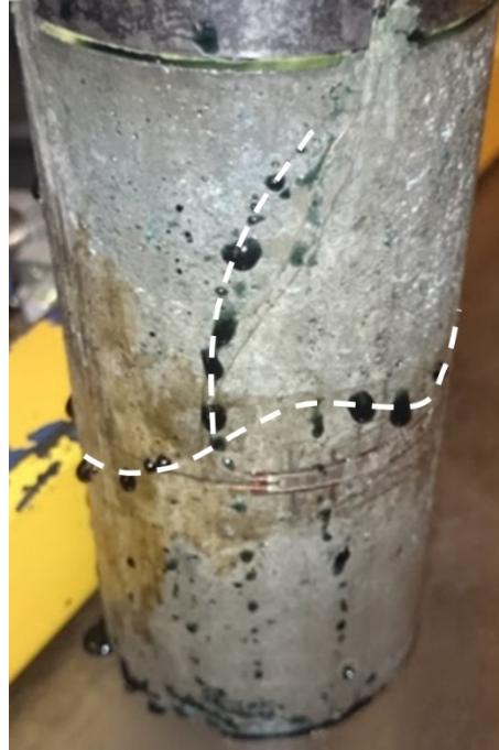
Fig. 23 Specimen number 24 with sub-horizontal and sub-vertical surface fractures under approximately 10 MPa hydrostatic remote stress conditions
