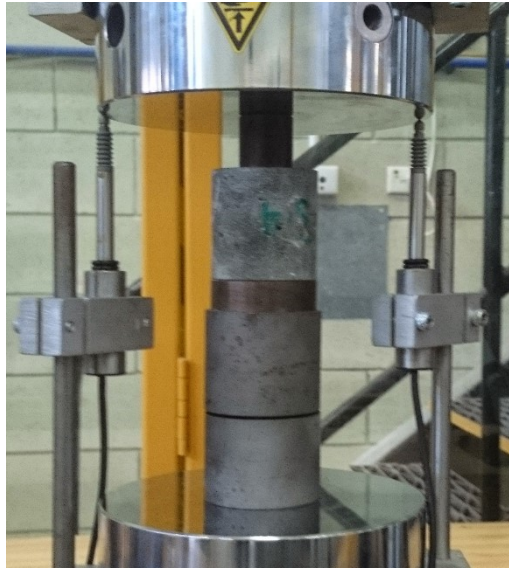
Fig. 7 Specimen setup before a punch through shear test was commenced
