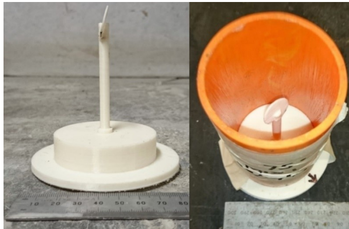
Fig. 1 Prototype mould of the 75° pre-existing circular notch
