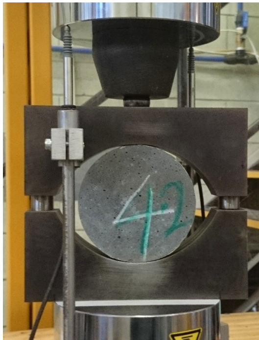
Fig. 4 Brazilian disc specimen before indirect tensile testing commenced
