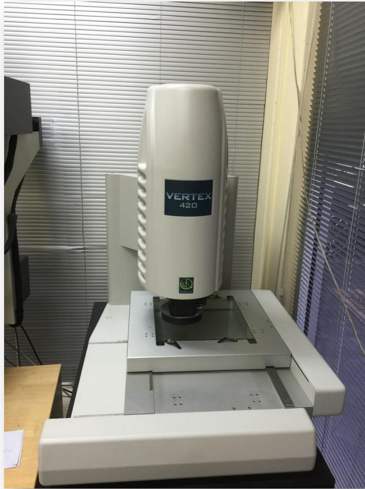
Figure 9: The automated Vertex 420 (Micro Vu, Windsor, USA), used for quantitative measurement of the Neoss implant replica, at Stoneglass Industries
