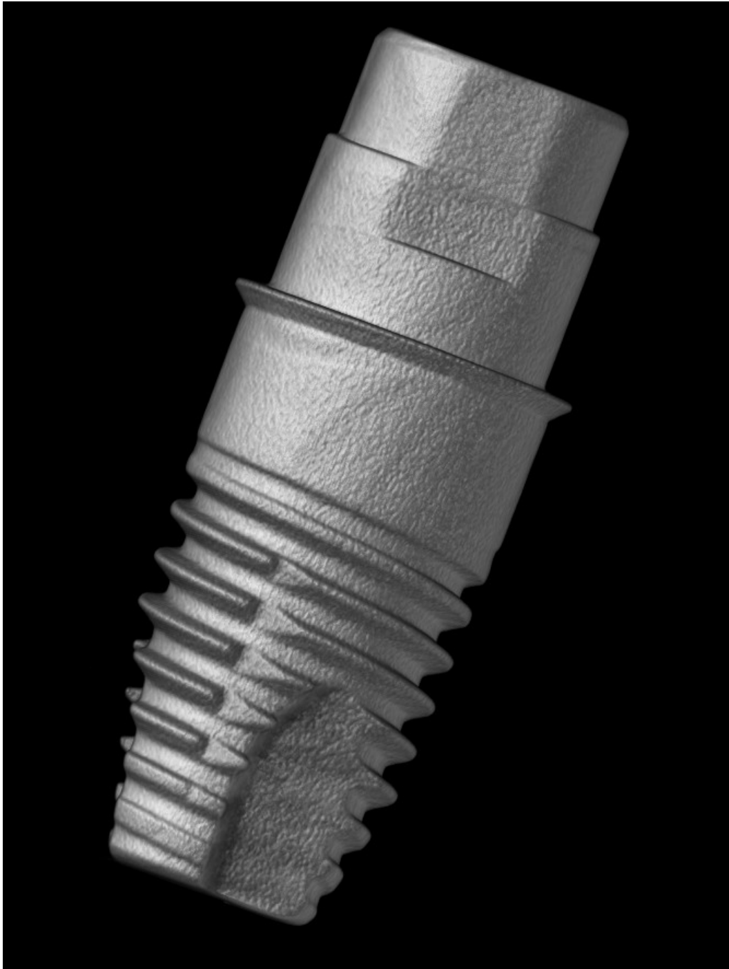
Figure 51: Specimen 3: External View 1 -- Neoss titanium NeoLink Mono attached to Neoss ProActive implant
