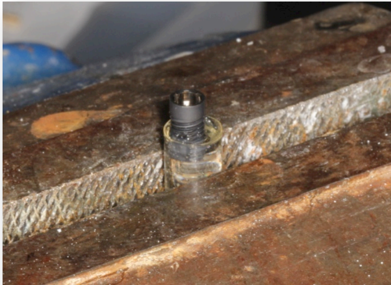
Figure 16: Neoss ProActive implant secured rigidly with epoxy resin in gelatin capsule. Specimen has been held in place with bench vice here, awaiting abutment insertion
