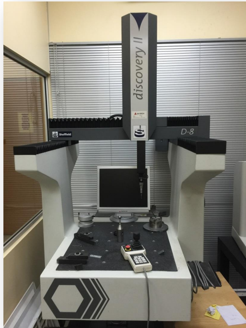
Figure 8: Sheffield Discovery coordinates measuring machine (Hexagon AB, Stockholm, Sweden) at Stoneglass Industries
