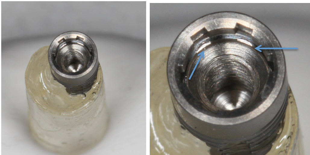
Figure 23: Specimen 4: Generic titanium abutment attached to Neoss ProActive implant. “Scuff marks” are evident on the internal aspects of the implant as indicated by the blue arrows
