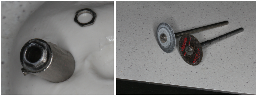
Figure 25: Specimen 4: Generic titanium abutment. The abutment had approximately half of its hexagon height cut off and polished with laboratory discs
