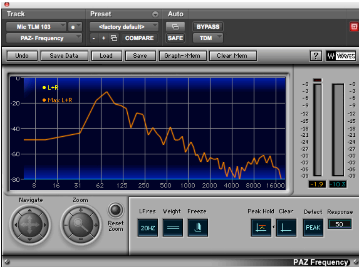
Figure 1.8 Frequency analysis C (65.41Hz). Sideways pulled, showing strong fundamental frequency registering minus 1.9 db from full scale, and relatively little high frequency information. (X axis represents frequency, Y axis represents amplitude, one-second duration).
