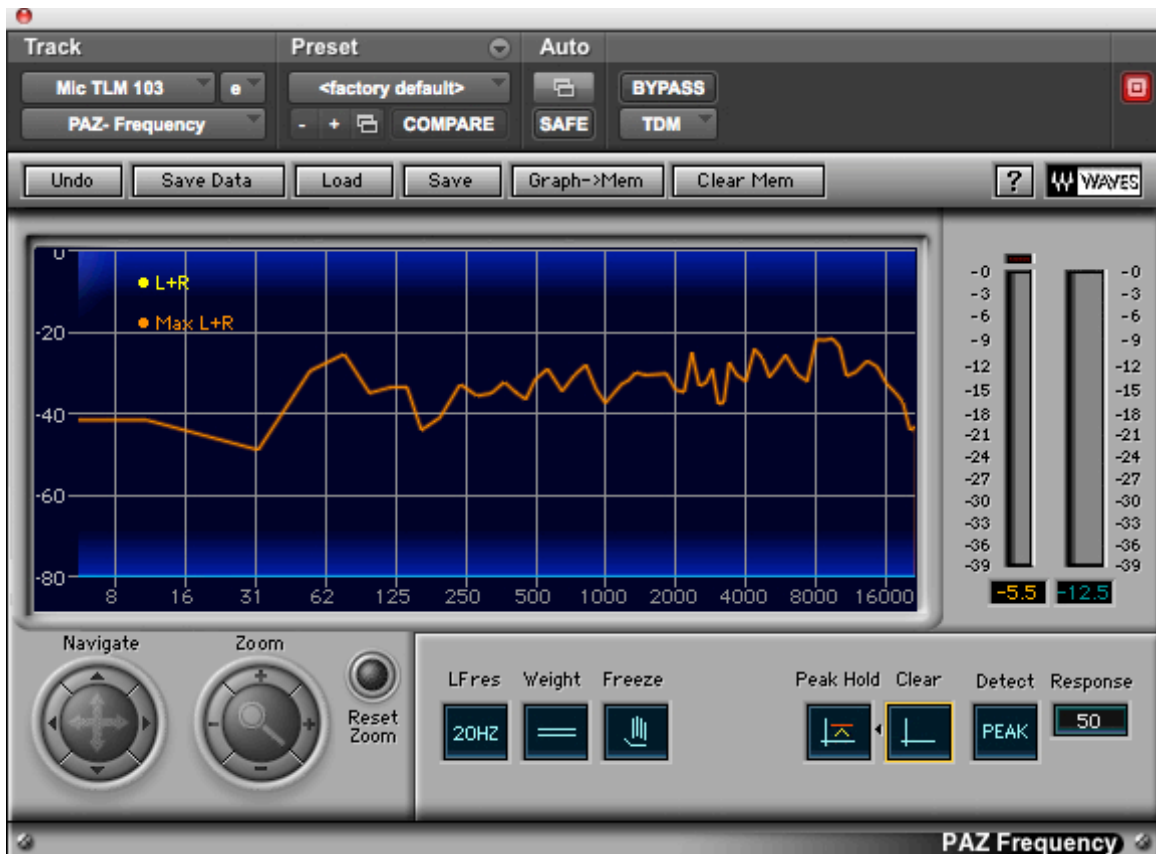
Figure 1.10 Frequency analysis C (65.41Hz) Slapped note displaying lower instantaneous volume (minus 5.5db), reduced fundamental, and greatly increased high frequency percussive component between 250Hz and 8kHz. (X axis represents frequency, Y axis represents amplitude).
