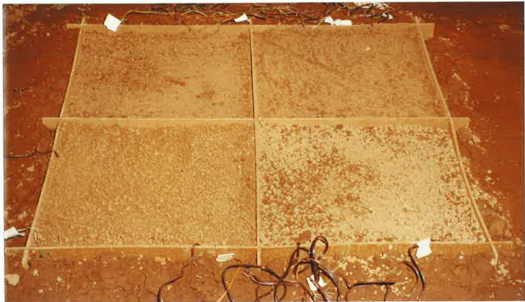
PLATE 6. Completed plot with thermistors and resistance blocks in place.
