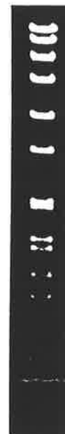
SPP-1 DNA/ Eco RI fragments. 0.5 \mu g/lane. 1% agarose gel stained with ethidium bromide.
