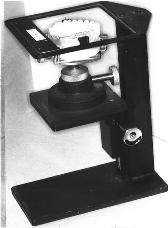
Figure 13. Device for adjusting height of occlusal plane prior to photography
