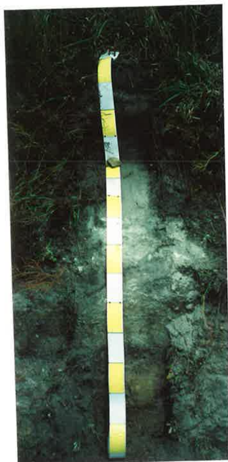
Profile (e) The Lucaston Sand photographed in a road cutting approx. 3 km from Profile (d). This is one of the few places where the siliceous hardpan (60 cm thick) has been penetrated. There has been some disturbance of the surface 20 cm of this profile.
