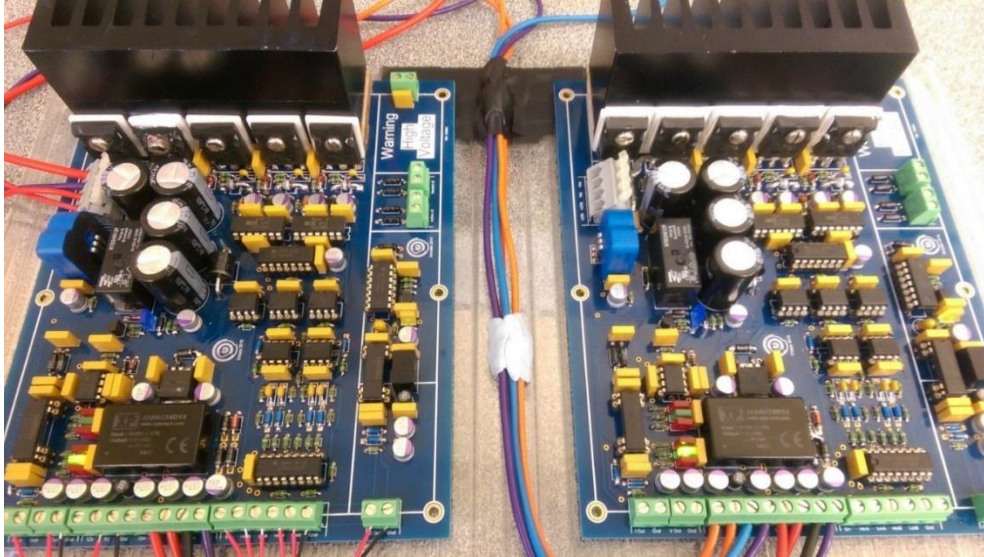
Fig. 6-22. Two completed MIC H-bridge PCBs undergoing testing.
