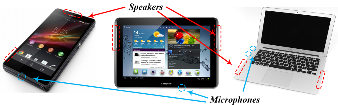
Fig. 8.2 Speakers and microphones in COTS mobile devices
