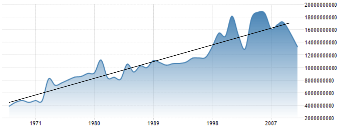
Figure 1.6: The losses (Kw.hr) of electric power transmission and distribution in Australia (World Nuclear Association 2016)
