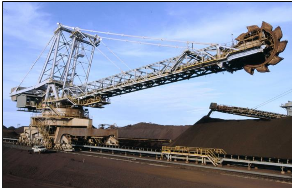
Figure 2.1: Bucket wheel reclaimer from ThyssenKrupp Robins
