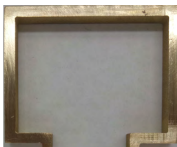
Figure 9.24. Topology of the cavity walls which are realized from a 3.2 mm thick section of brass.
