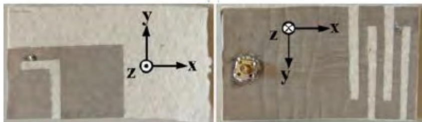
Figure 2.32. A dual-band slot loaded PIFA for operation at 433 MHz and 2.4 GHz as reproduced from [27].
