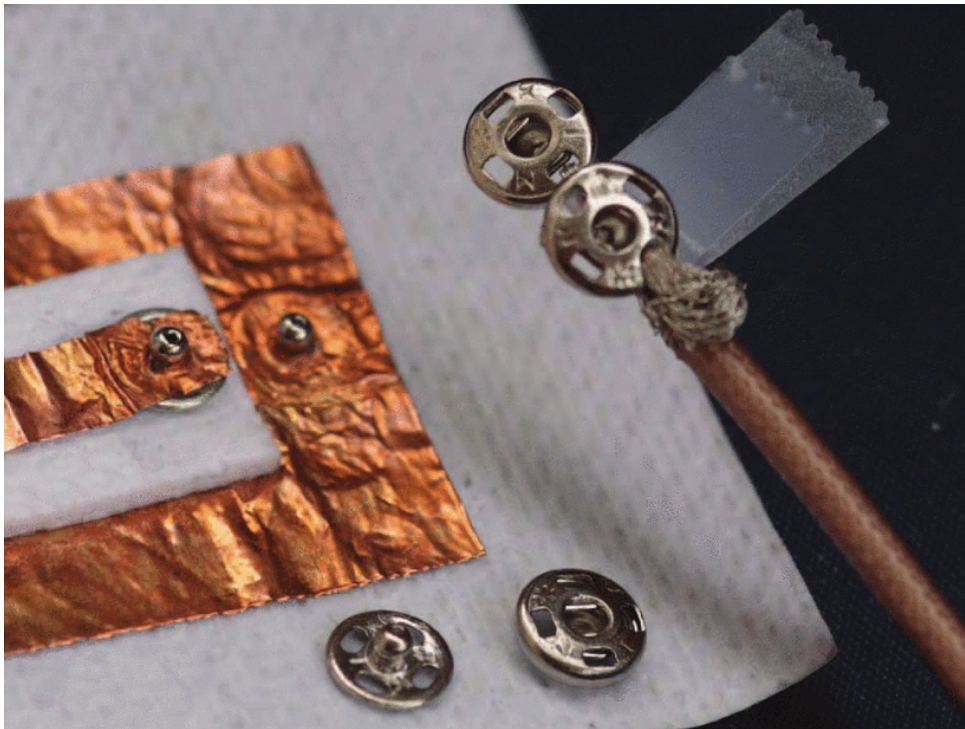
Figure 3.4. Commercial snap-on buttons used as a replacement for a SMA connector in a textile microstrip line as reproduced from [42].
