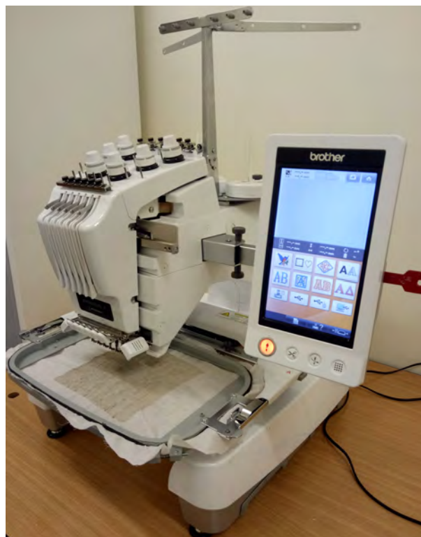
Figure 2.9. A computerized embroidery machine that can be used for the realization of textile antennas.
