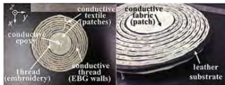
Figure 2.38. A patch antenna periodically loaded with a EBG structure for surface wave enhancement as reproduced from [33].
