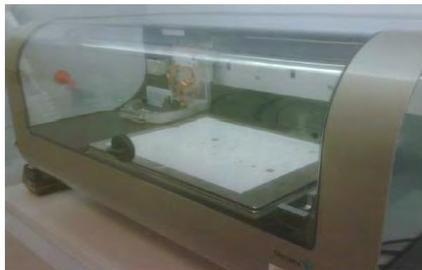
Figure 2.4. A typical inkjet printer that can be used in the realization of flexible microwave devices. This image is reproduced from [4].
