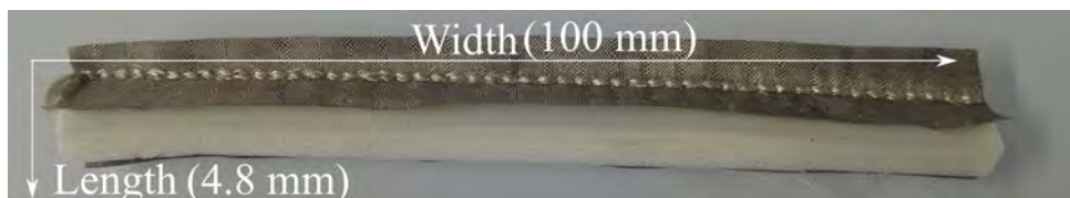
Figure 6.8. A section of an embroidered wall used to obtain a effective frequency dependent sheet resistance.
