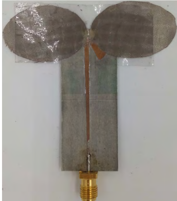
Figure 2.6. A wideband dipole antenna patterned from a conductive fabric. The textile dipole is excited through a balun which has been fabricated from Rogers Duroid 5880.
