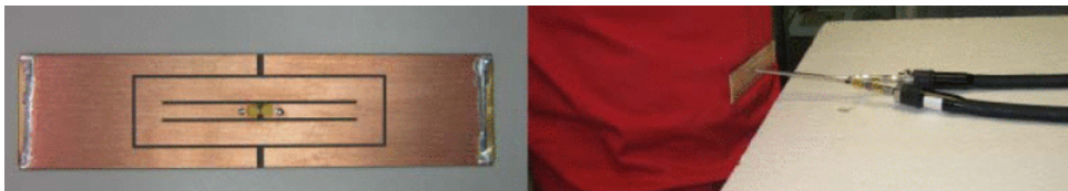
Figure 6.1. A broadband UHF antenna suitable for on-body operation as reproduced from [51].
