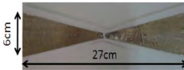
Figure 2.22. A textile bow-tie dipole antenna as reproduced from [18].
