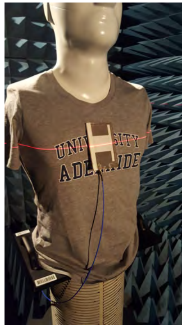
Figure 6.19. Measurement setup for the radiation patterns of the antenna when in close proximity to body tissue which is approximated here by a human body phantom.
