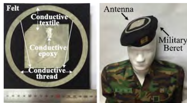
Figure 2.31. A dual-band textile antenna exploiting two independently fed radiators with omni-directional and broadside radiation patterns for integration into a military beret as reproduced from [26].
