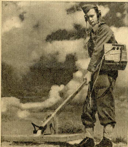
A sapper goes into action as a land mine sweeper. He is using as a detector a grid attached to a pole. The grid is connected electrically with the earphones.
