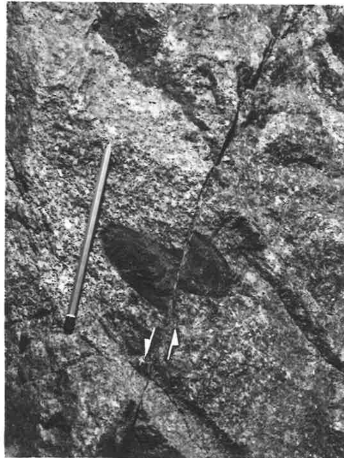
PLATE 9. Relative movement of adjacent joint blocks in granite, indicated by the displacement of a xenolith.
