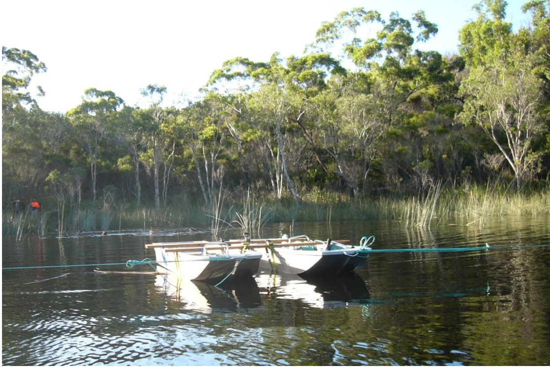
Figure 9: The coring platform, constructed from two 3.75 m tin boats sits above the location of core SL/15-1. Photo by J. Greer
