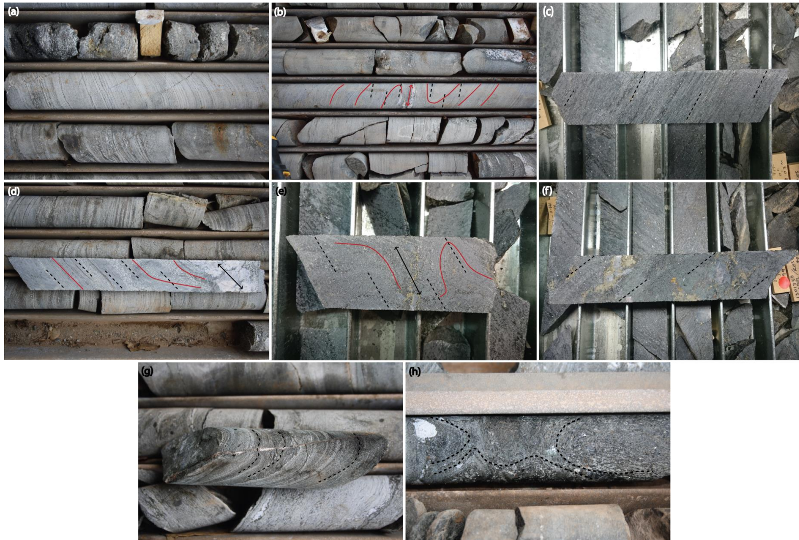
Figure 4: Representative drill core from DDH 114 and DDH 200; a) unaltered metasediments with small fractures offsetting planar compositional banding; b) unaltered metasediments containing folded compositional banding with fine grained biotite foliation axial to fold hinges and thin 1cm pegmatite intruding along foliation; c) moderately altered metasediments dominated by medium grained biotite foliation; d) moderately altered metasediments containing folded compositional banding cross cut by large pegmatite which intrudes along foliation; e) highly altered metasediments containing hematite alteration with pegmatite and sulphide mineralisation along foliation; f) highly altered metasediments with sulphides developed along foliation axial to fold plane; g) highly altered metasediments with hematite/pegmatite vein cross cutting and locally folded coarse-grained biotite foliation; h) highly altered metasediments with disrupted pegmatite and an intense biotite shear zone in which the foliation has been folded by a later event.
