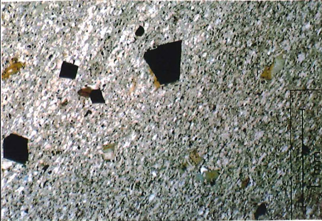
a: Fine grained Ulupa Siltstone within the zone of shearing. Large euhedral porphyroblasts of magnetite are observed randomly in the fine mica-rich matrix. Other small opaque grains of rutile are observed.
