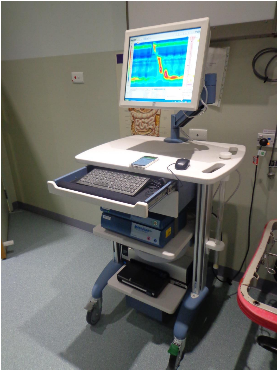
Figure 2-17 Hardware and software for recording and analysis from a solid state catheter.
