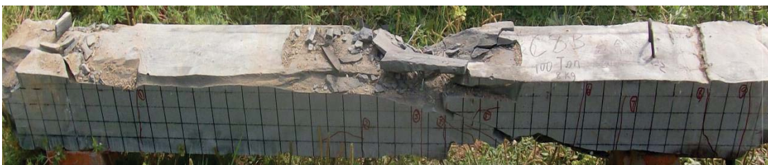
H2B Specimen with 1000 kN axial load under 8 kg charge weight loading
