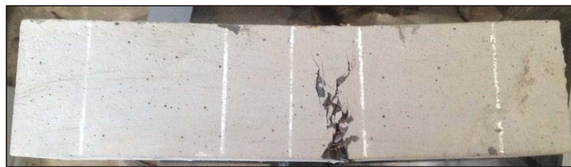
(b) Failure of UHPC specimens
