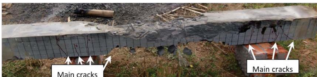
(b) H7A Specimen with no axial load axial load under 24 kg charge weight loading
