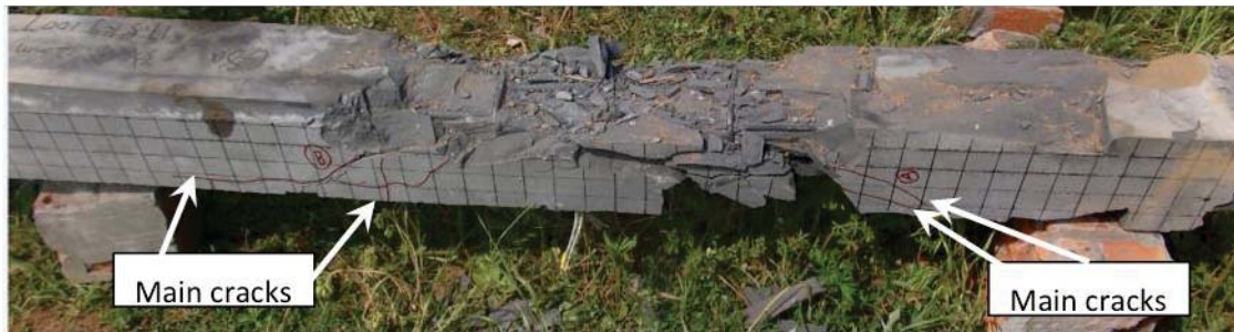
(d) H8A Specimen with 1000 kN axial load under 24 kg charge weight loading
