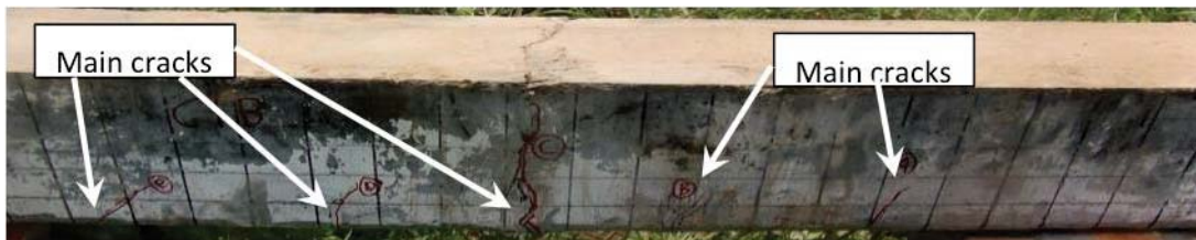
U1B Specimen with 0 axial load under 17.5 kg charge weight loading
