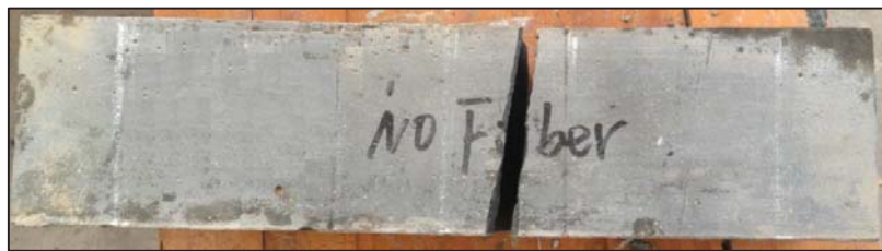
(a) Failure of high strength concrete specimens
