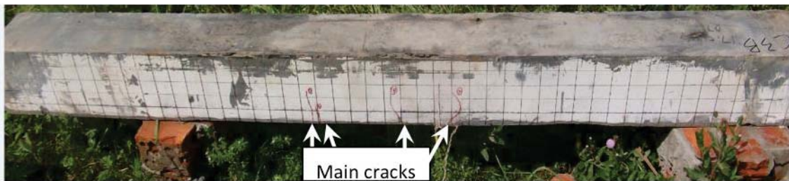
(a) U3B Specimen with no axial load under 24 kg charge weight loading
