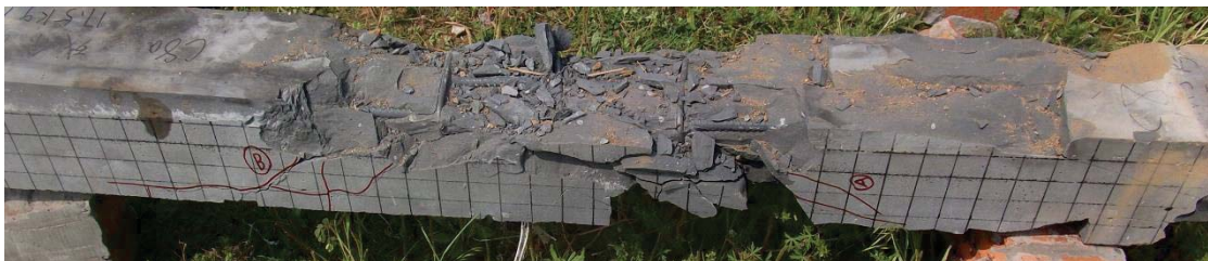
H2A Specimen with 1000 kN axial load under 17.5 kg charge weight loading
