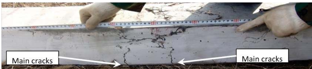
U1B Specimen with 0 axial load under 17.5 kg charge weight loading
