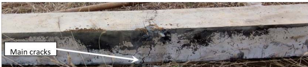
U1A Specimen with 0 axial load under 35 kg charge weight loading
