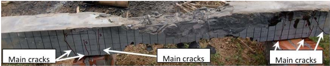
H1A Specimen with 0 axial load under 17.5 kg charge weight loading
