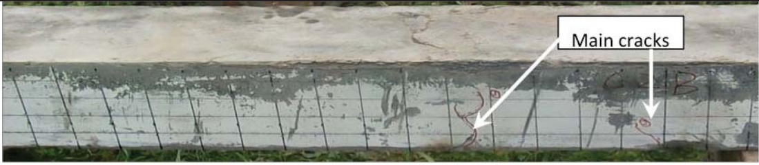
U2B Specimen with 1000 kN axial load under 17.5 kg charge weight loading
