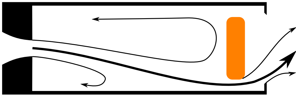
Figure 2.6: Streamlines of the FPJ flow that deduced based on the measured phase-averaged axial velocity. Adapted from Wong et al. (2004).
