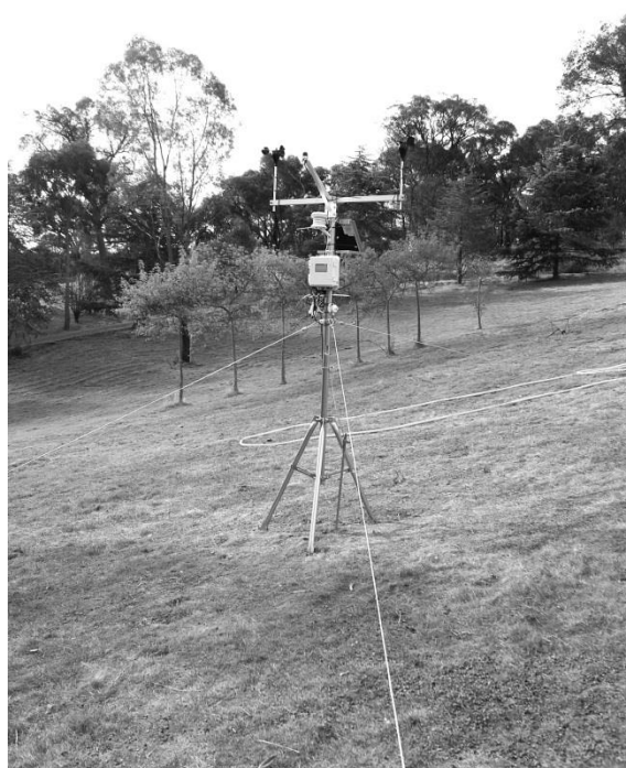
Figure 3.4. HOBO U30 weather station, Nillumbik Shire
