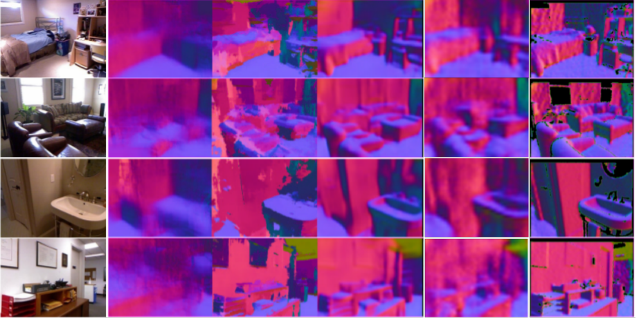
Figure 3.11: Comparison of different surface normal prediction methods against our proposed fast architecture. From left to right are: (1) the input image, (2) normals from Fouhey et al. [2013], (3) normals from Ladický et al. [2014], (4) normals from Eigen and Fergus [2015] that are used for all our experiments, (5) normals from our fast but less accurate model proposed in this section, and (6) groundtruth normals computed from Kinect depth data.
