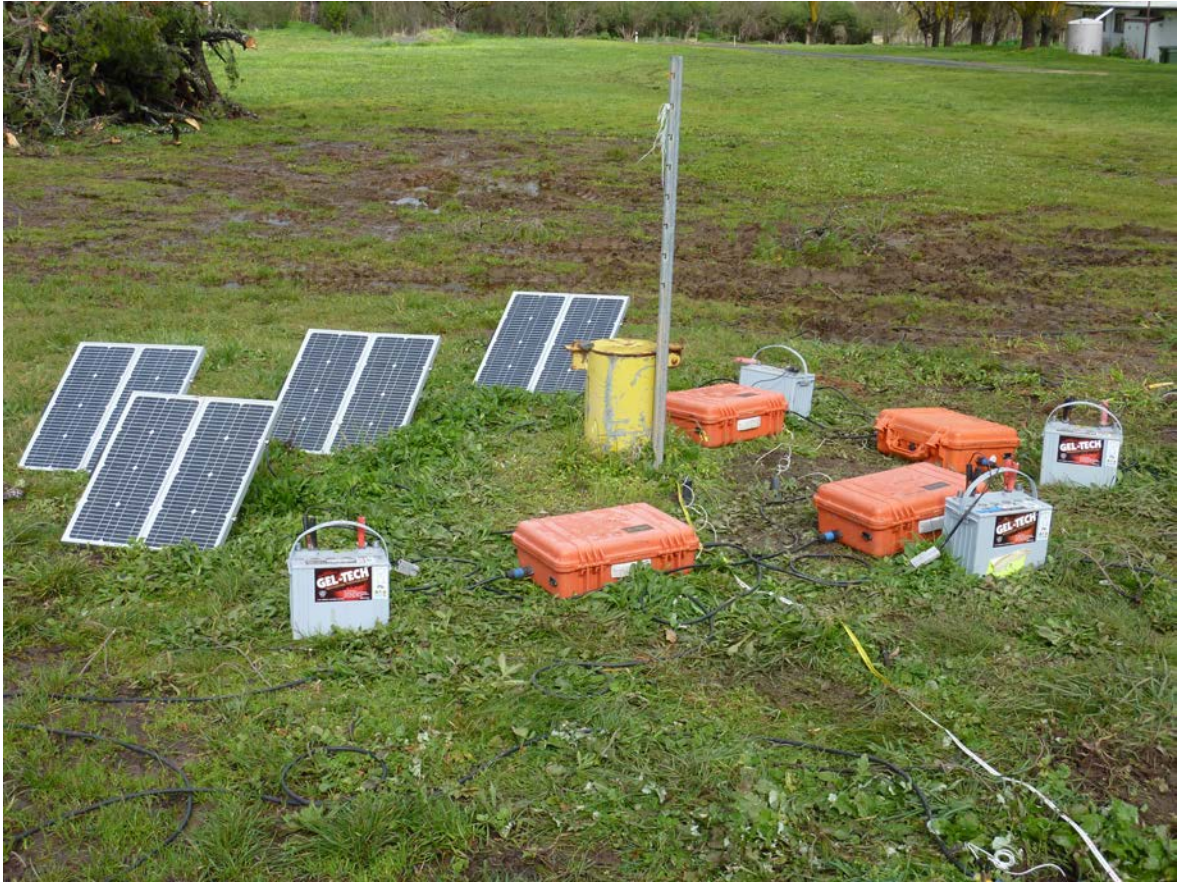
Figure 3.4: A field photograph of the University of Adelaide SP Instrument setup at the pumping well in Watervale, Clare Valley, South Australia.
