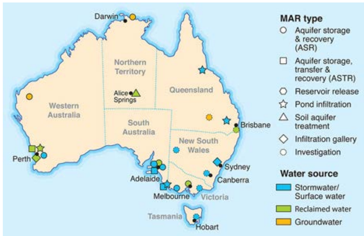
Figure 6.2: Stormwater aquifer storage and recovery (ASR) scheme locations around Australia. In South Australia ASR schemes supply approximately 20 GL/yr of groundwater recharge. Recharge estimations of 60 GL/yr are expected by 2050. Figure from CSIRO: Managed aquifer recharge scheme (2017).
