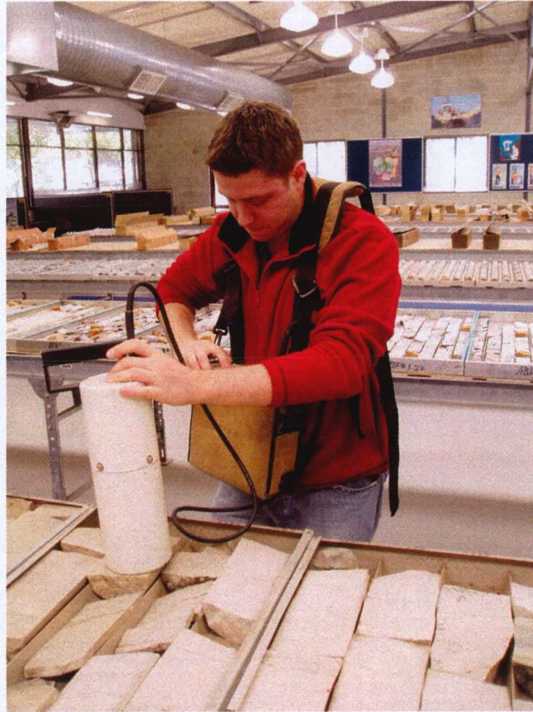
Figure 3.1 Acquisition of core spectral gamma ray data
