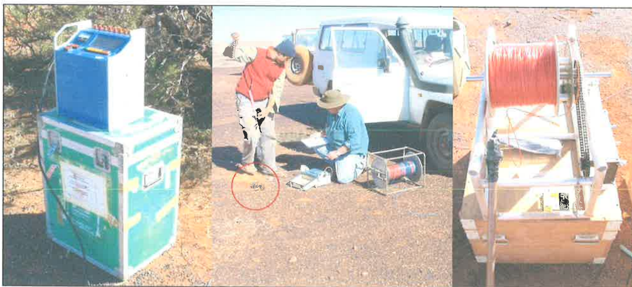
Figure 3.46: (left) IRIS VIP 4000 transmitter capable of delivering 4KW of power. (middle) ELREC 6 receiver, PPE/1 porous pot (circled) and operators at a measuring station. (right) Crone DHEM hand winch with cable reel and electrode attached and ready to deploy.
