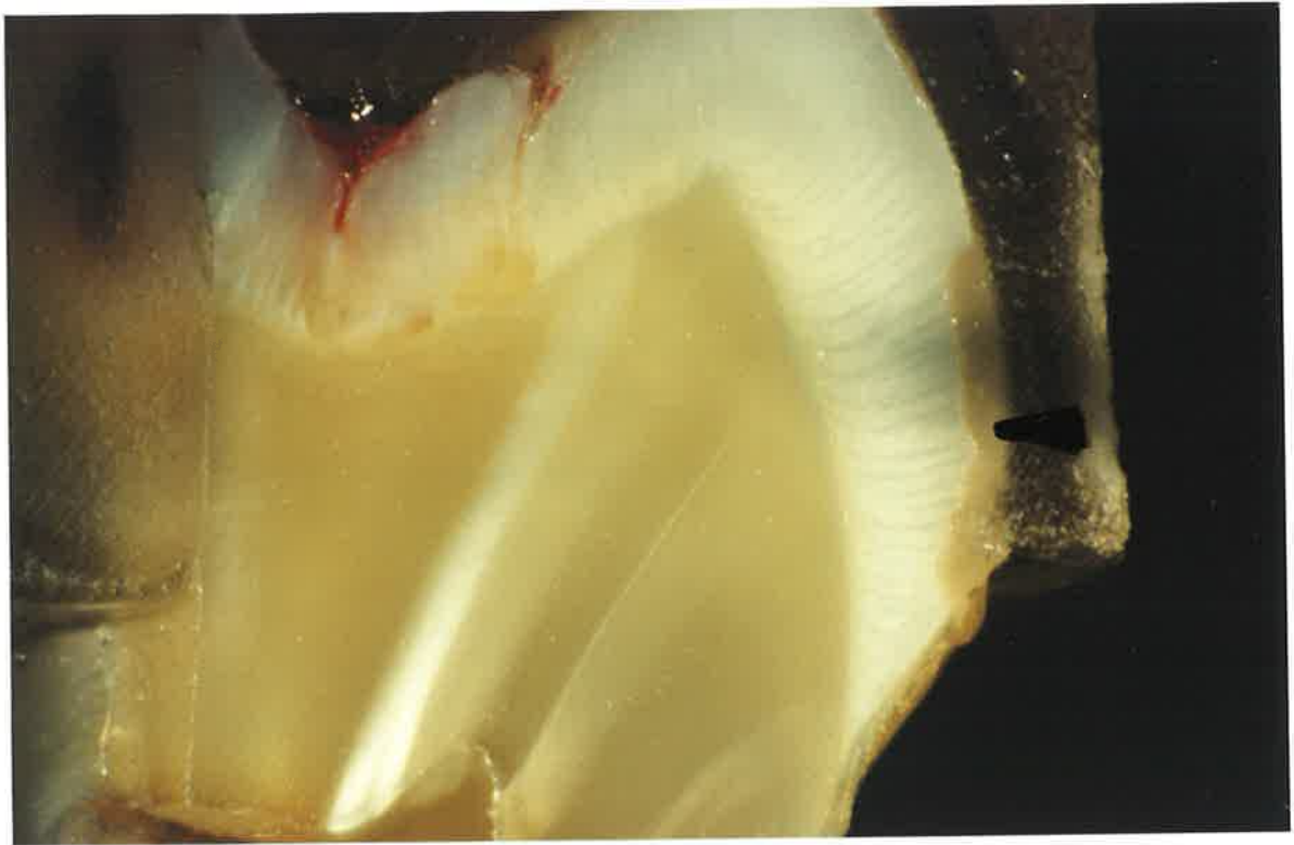
Figure 36(a). Cross-section of selected control specimen from 4-minute "cyclical erosion" model showing depth of erosion reached after 192-228 cycles of exposure time to test solution.
