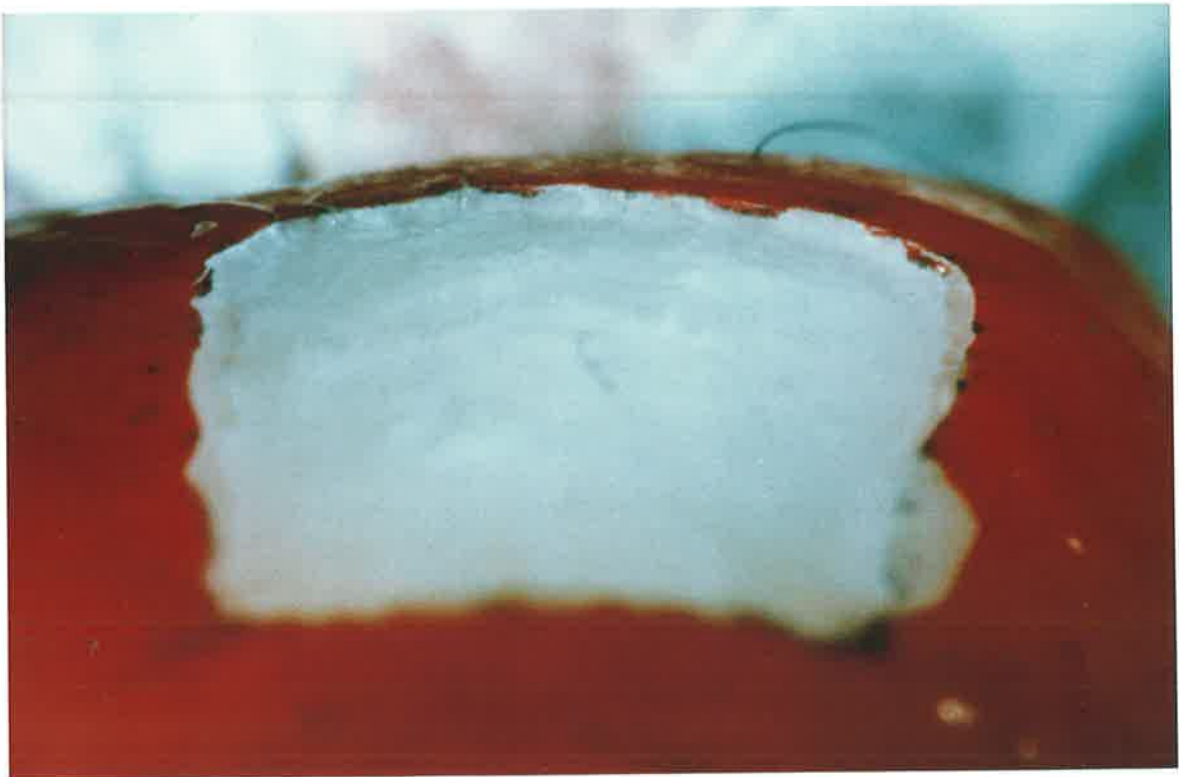
Figure 30. Example of a specimen showing 0.25mm depth loss (sample tipped to show semi-profile view of margin of lesion).
