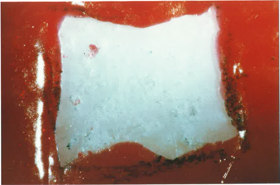
Figure 29. Example of a specimen showing total surface etch.
