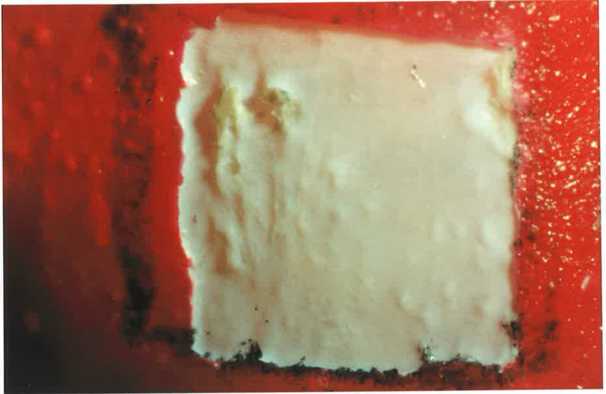
Figure 9. Representative specimen following exposure to test solution for 2 hours (a) Showing irregular surface of erosion lesion. (b) Cross-sectional view showing depth of erosive lesion.
