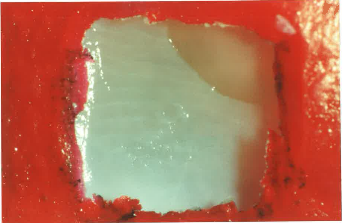
Figure 13. Representative specimen following exposure to test solution for 18 hours (a) View of surface of erosive lesion. (b) Cross-sectional view showing depth of erosive lesion.
