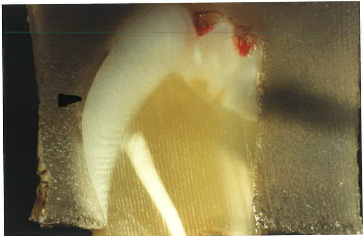
Figure 36(b). Cross-section of corresponding test specimen showing effect of fluoride in inhibiting progress of erosion for the same exposure period to the test solution.
