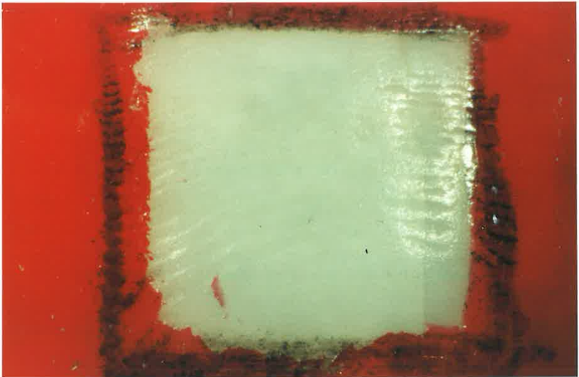
Figure 4. Example of a prepared specimen prior to exposure to erosive solution (x20 magnification).
