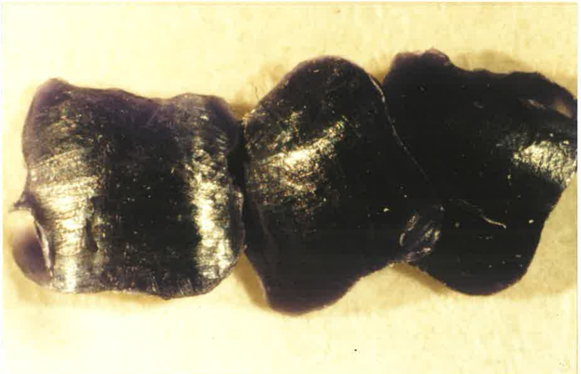
Figure 7. Three completed wax patterns for the one specimen.
