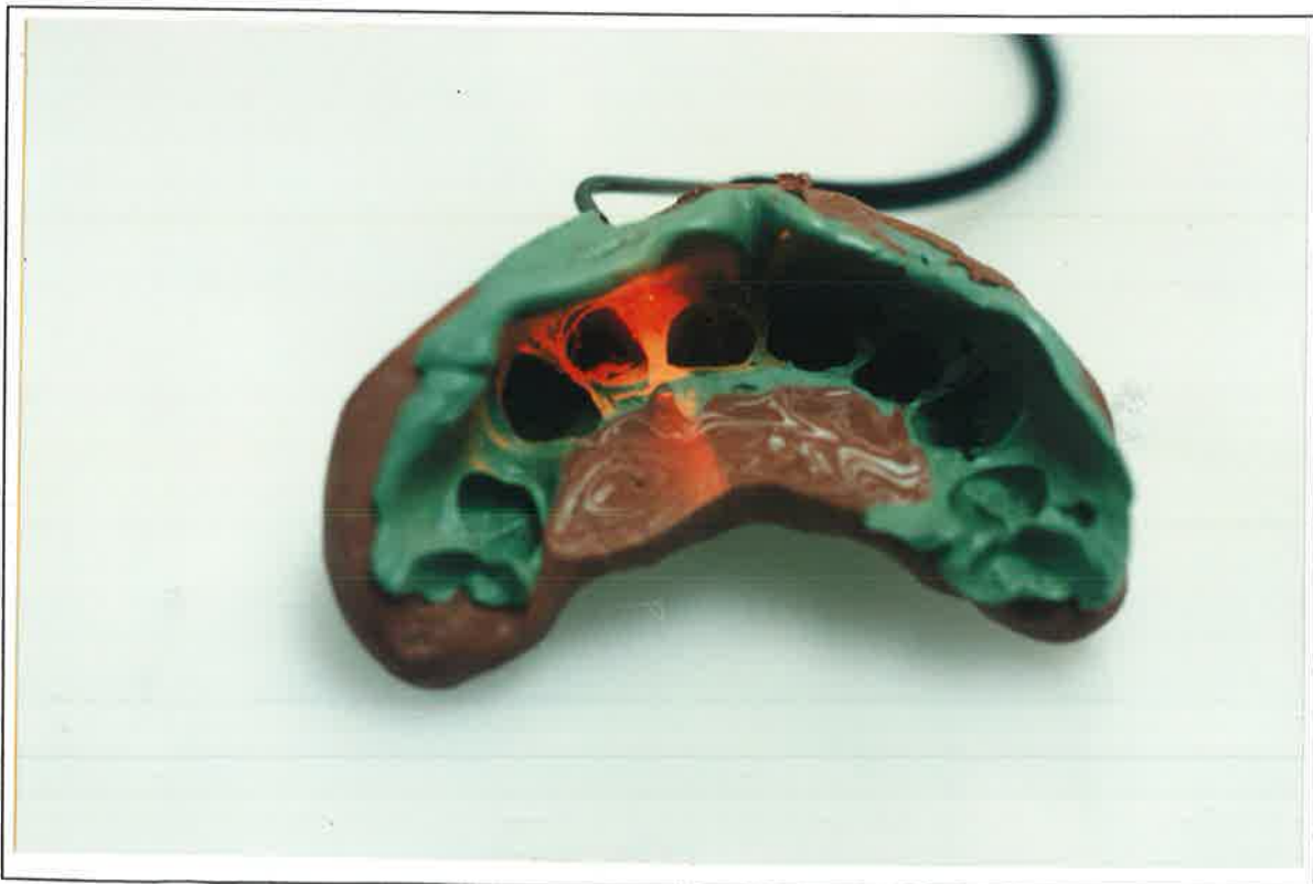
Figure 4: Custom stent for stabilising and accurately positioning probe. The green polyvinylsiloxane material (Kerr Extrude) partially absorbs scattered light and minimised light scattering to and from the gingiva.
