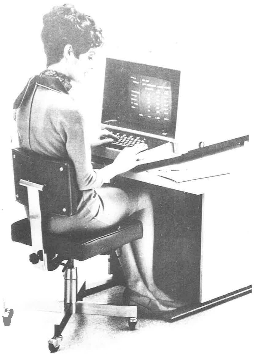
Figure 3. Remote computer terminal showing teletype keyboard and VDU
