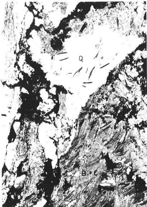
a) TS 4364. Quartz segregation in biotite-chlorite schist. Where quartz is in contact with chalcopryrite it has curious lobate margins, possibly indicating replacement by chalcopryrite.
