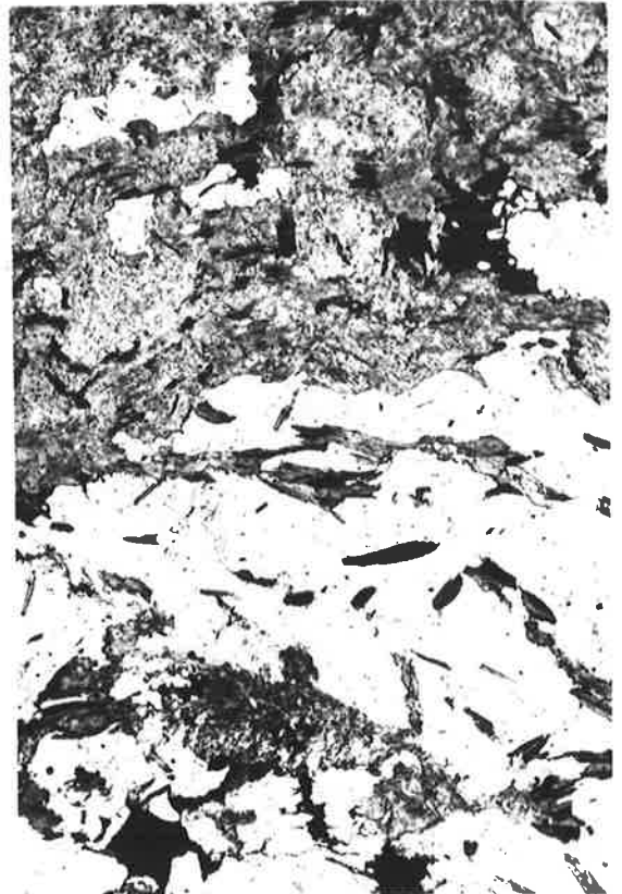
b) TS 4365. Banded mica schist. The upper band is composed of sericitic muscovite, biotite and chlorite with minor quartz and chalcopryrite. Lower is predominantly quartz.
