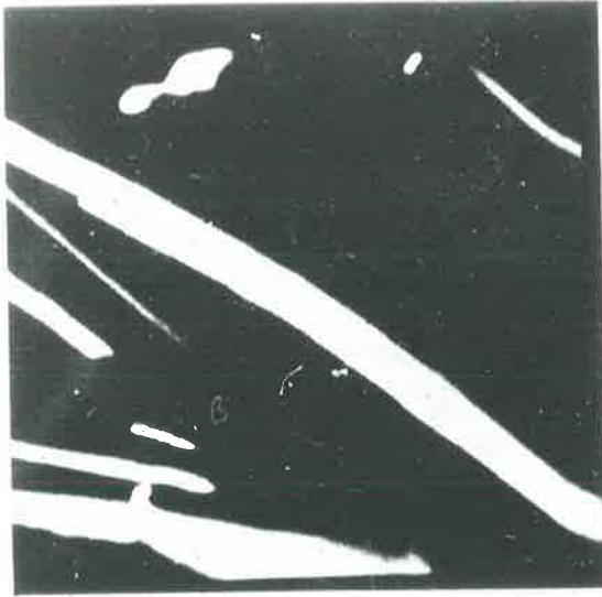
Secondary electron image showing grain shape
