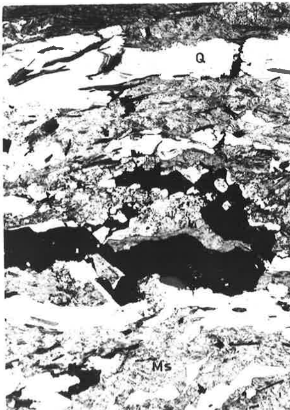
c) TS 4367. Sericitic muscovite, biotite & chlorite intergrown with quartz & opaques.
