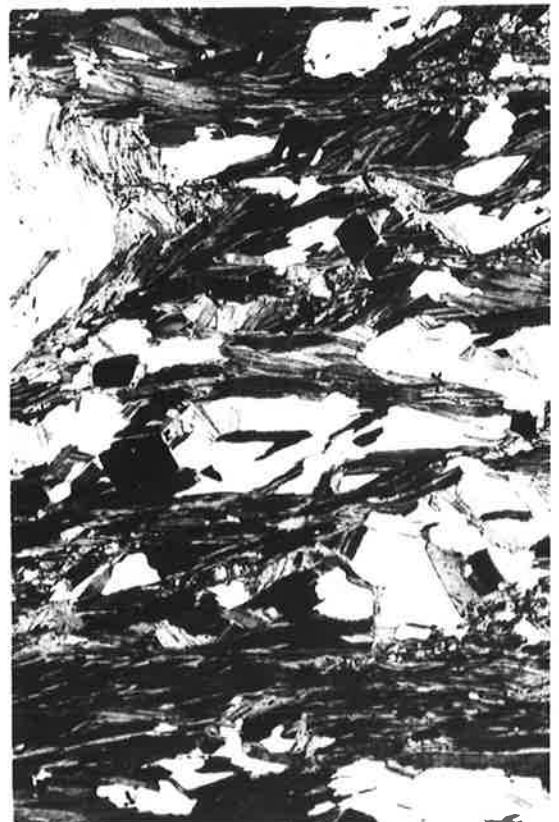
d) TS 4368. Well-developed schistosity defined by sub-parallel biotite, chlorite & muscovite.
