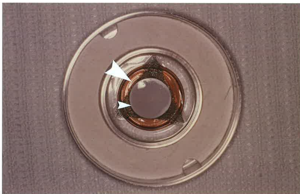
Figure 2.2 - Testing assembly II Inner well with labelled medium (large arrow) contacting cells on filter (small arrow)
