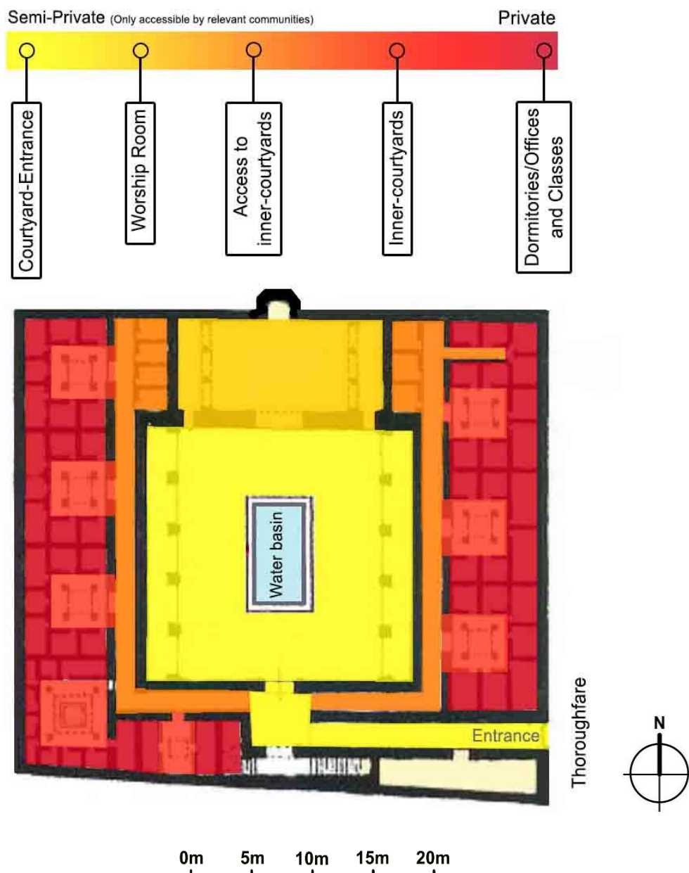
Figure 3.14: Hierarchical conditions as a result of the application of semi-public in-between spaces, in a historic city could have generated social grouping within neighbourhoods. Basic drawing (the Ibn Yusuf Madrasa) in Morocco, courtesy of Kamiya (2004)
