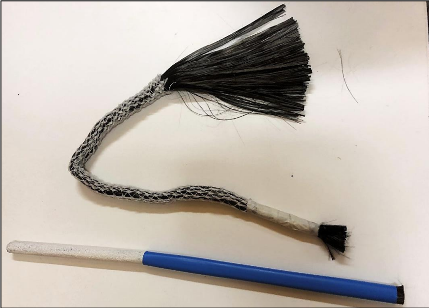
Figure 1. Examples of a dry anchor at the top and a partially pre-cured anchor at the bottom
